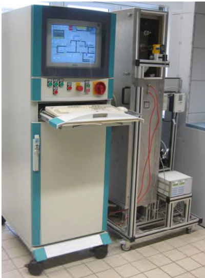
Figure 3.3: Front view of the equilibrium adsorption apparatus with insulation shell removed, the yellow pyrometer and its control unit
