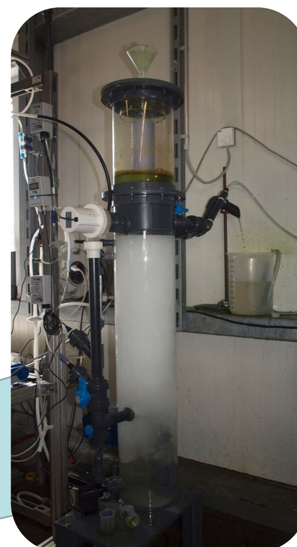
Harvest of algae with ozone-enhanced flotation; The flotote has a biomass concentration of > 60 g/l. The clarified culture medium is send back to the RAS.
