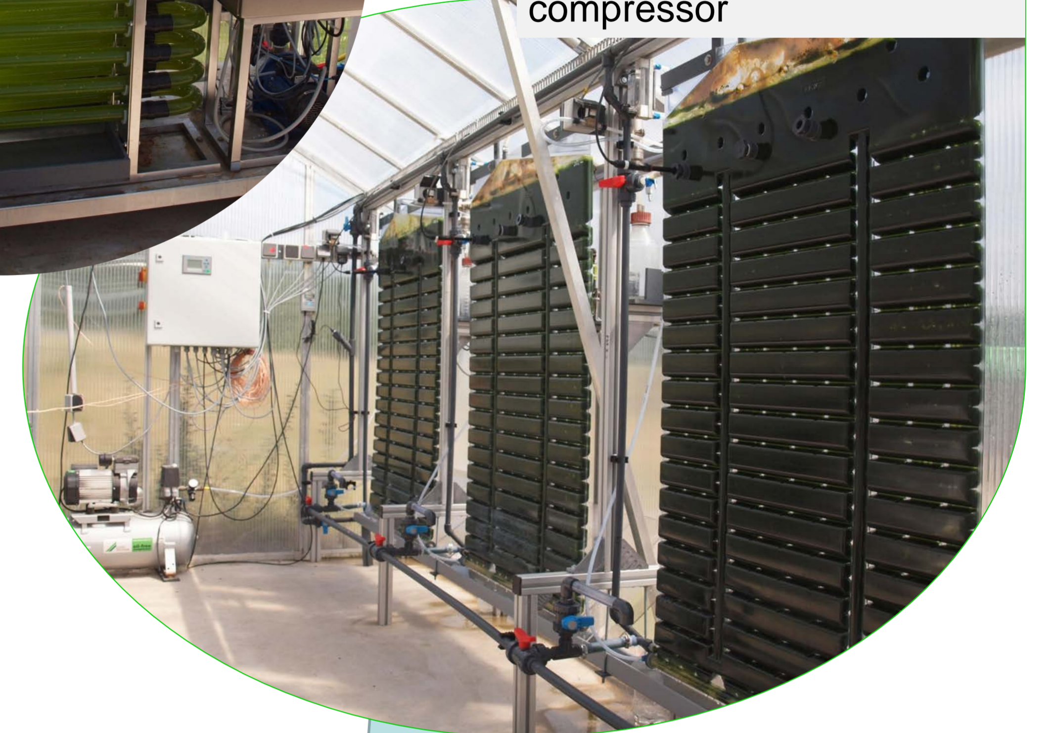
Flat panel airlift PBR (Subitec GmbH); 3 x 25L Background: PLC, compressor
